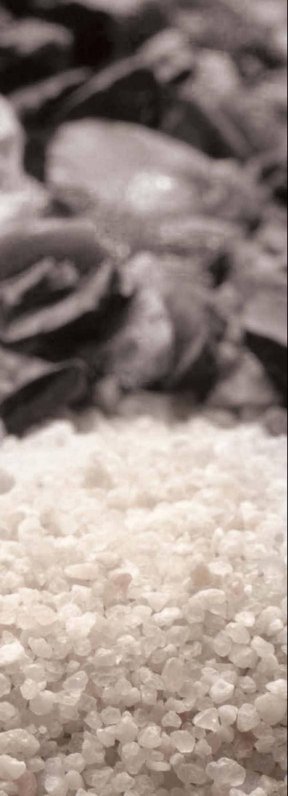
TechniStone® is made from natural materials (quartz and granite) and a high-quality binding agent, supplemented with coloured pigments and glass or mirror granules. In the form of highly durable large-size boards, hardened stone is widely used in the private, public and industrial sectors.
