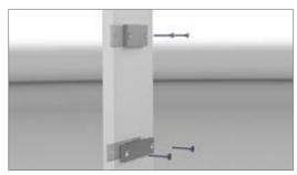
Fix base plate at the basic substructure
