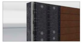
Mount the T-profile with approved fastening means
