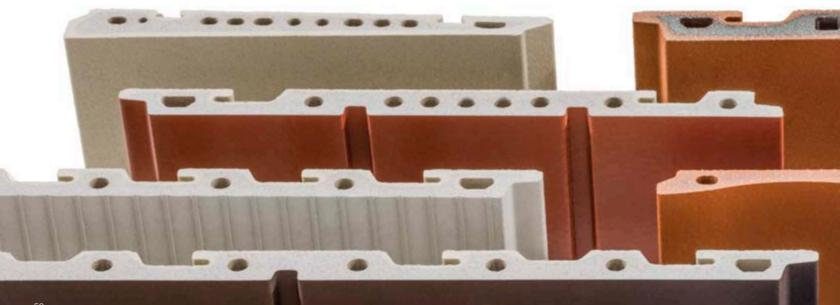
Extruded Ceramic Panels, Precision, DIN EN 14411, group Alla, glazed/unglazed (GL/UGL) (small-/large-size stoneware panels), 20 mm thick, 32 kg/m<sup>2</sup>
